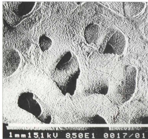
Fig. 1 Electron Microscopy of Porites Porites coral showing pores ranging from approximately 80 to 120 microns in diameter, interconnected in a trabecular pattern.
